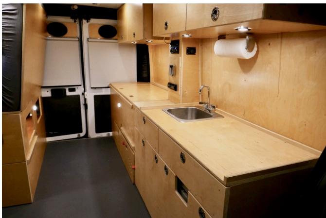
Raise the Murphy bed (left) and the MUV is transformed into a hauler or a mobile office for interacting with clients
